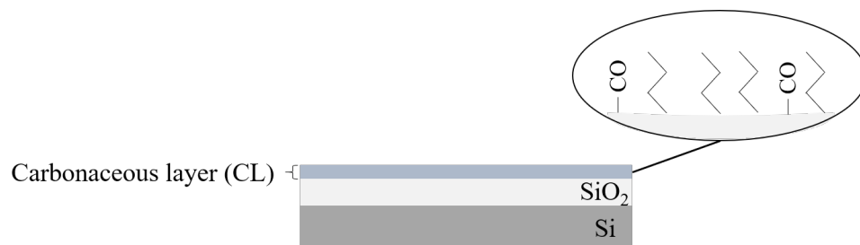
Figure 4.18: Carbonaceous layer formed on top of SiO 2 thin films due to film aging.
